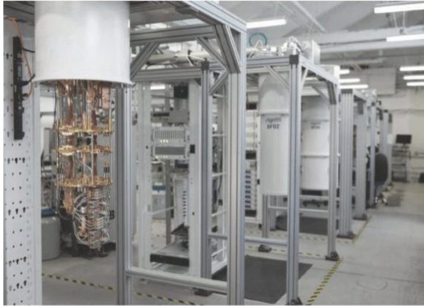
Rigetti's quantum computing facility in Berkeley, California includes both research and development and production quantum processing units, which are each housed in a cryogenic refrigerator.
