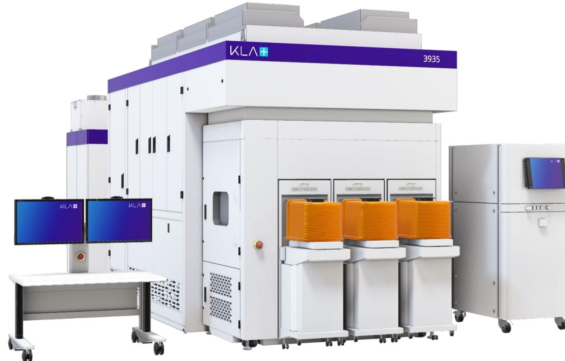
(Top) The 39xx Series “GEN 5” has played a critical role in defect discovery for advanced devices and in the transition to EUV lithography.
