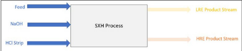
Figure 10-9: Diagram of the SXH Process
